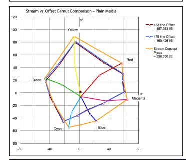
The significantly larger gamut volume of Stream prints relative to both 133-line and 175-line Offset on both plain and glossy media opens the potential (some of which has not yet been achieved) for printing richer photographs and documents with higher impact than Offset.
