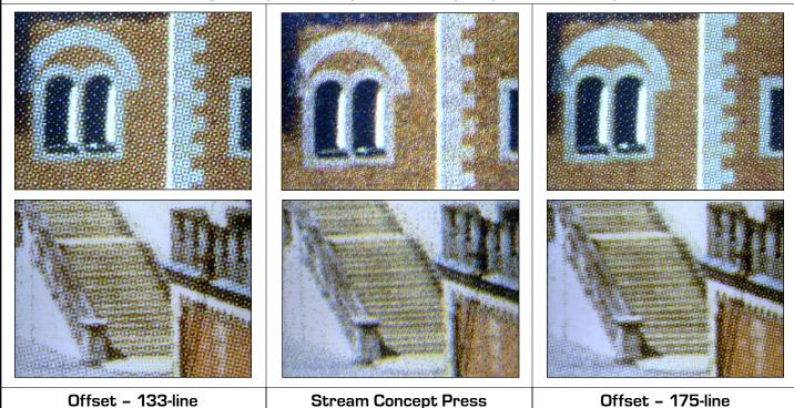
on Stream prints on dull and plain media. Screening patterns were visible on both Stream and Offset prints, particularly on high coverage areas on coated media, thus detracting from overall print quality appearance; this added a grainy and soft appearance on Stream while showing a distracting rosette pattern on Offset, especially at 133-line.
